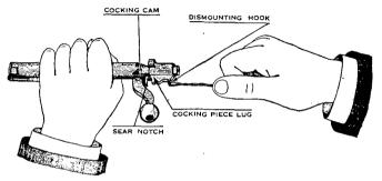
FIGURE 6.-Withdrawing cocking piece.
